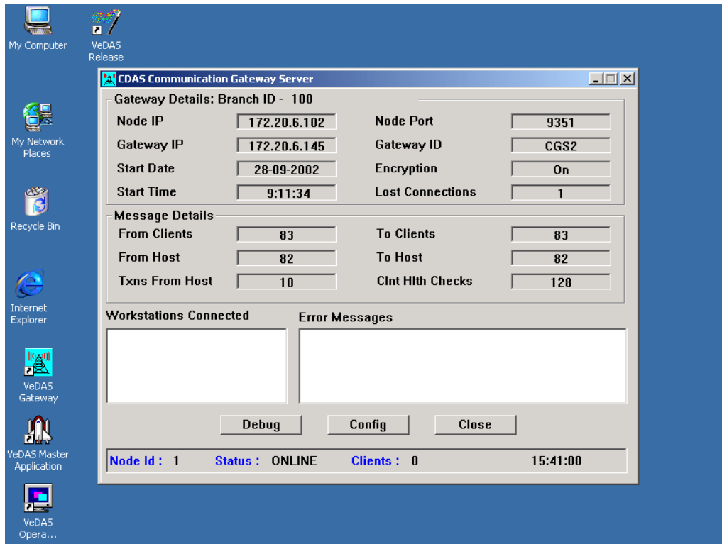
Figure 2.3. Communication Gateway Server application started by double-clicking the VeDAS Gateway icon on the desktop
