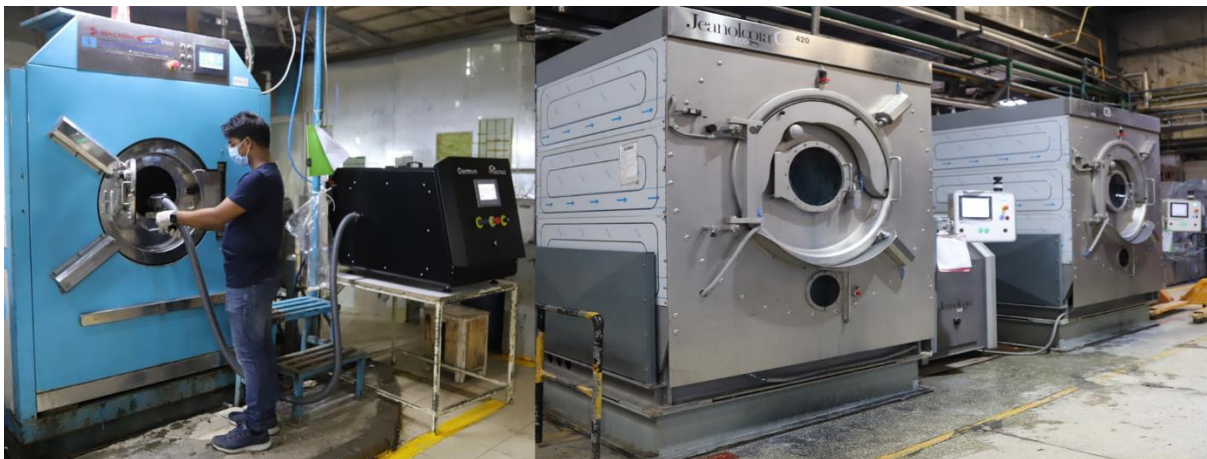
1:1 liquor ratio for water saving and uniform application of chemicals
